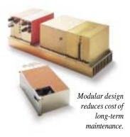
In-The-Field Reliability is ensured by ETM's rigorous testing program. Every ETM amplifier is subject to an environmental burn-in that includes temperature cycling, multiple cold starts from -20°C, and, as required, shock and vibration testing.
